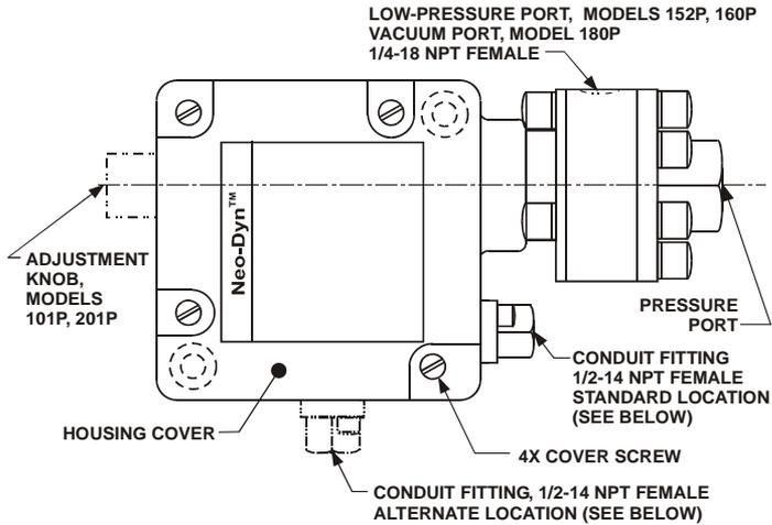
Figure 1: Models 100P, 101P, 110P, 142P, 152P, 160P, 180P, 200P, 201P: Enclosure 3X Adjustable Pressure Switches (Pressure Port Configurations Vary with Model and Range)
